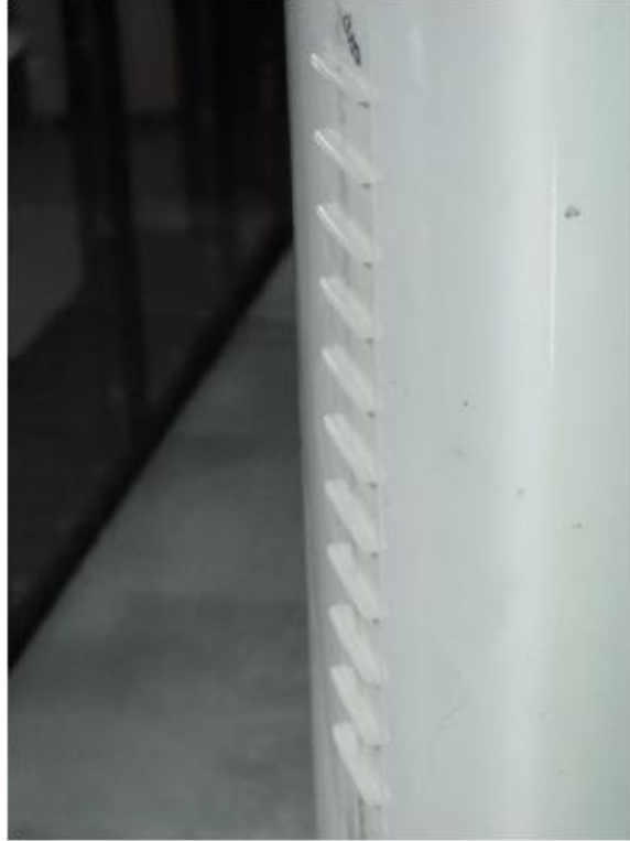
Figure 10. Boundary layer trip fitted on the Wind turbine blade section model (3/4 view as seen from upstream)
