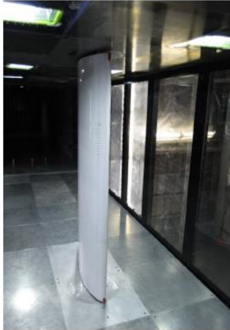
Figure 8. Wind turbine blade section model fitted with boundary layer trip (overall view)
