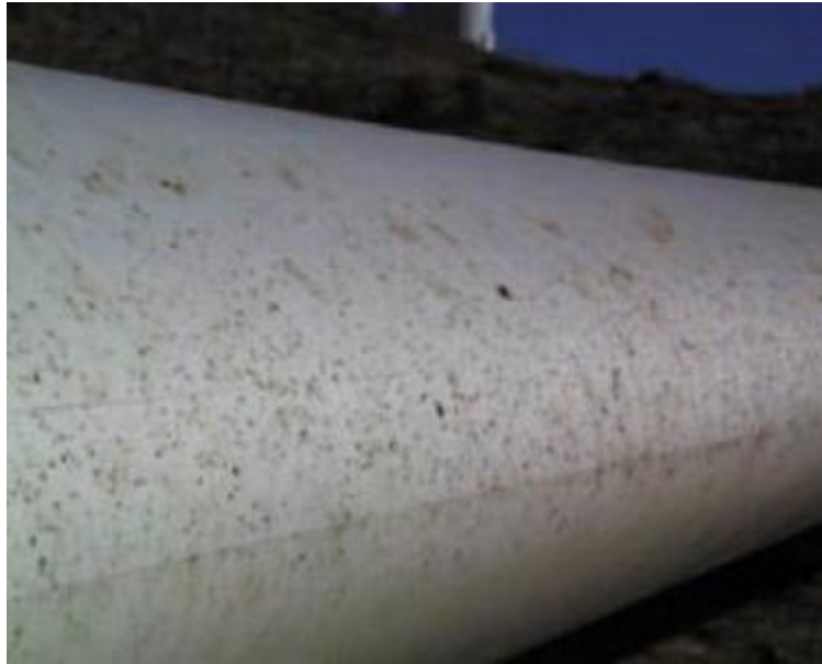
Figure 1. Insect accumulation on the leading edge of a wind turbine blade (Dalili et. al. , 2009)
