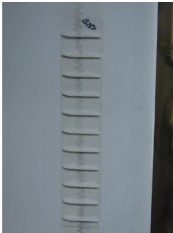
Figure 9. Boundary layer trip fitted on the wind turbine blade section model (side view)
