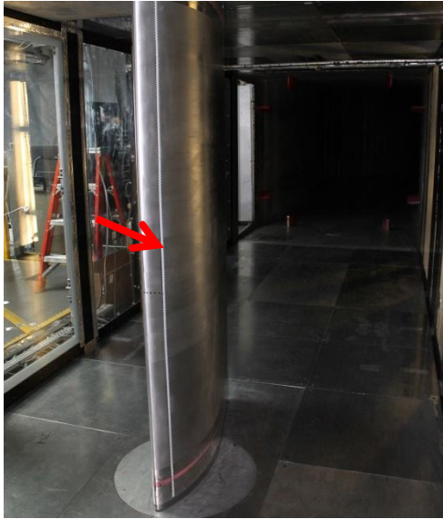
Figure 4. Trip applied near the leading edge of an airfoil. The trip strip is indicated by the red arrow.
