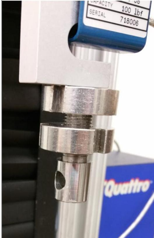
Mount lower adapter to load transducer and tighten
