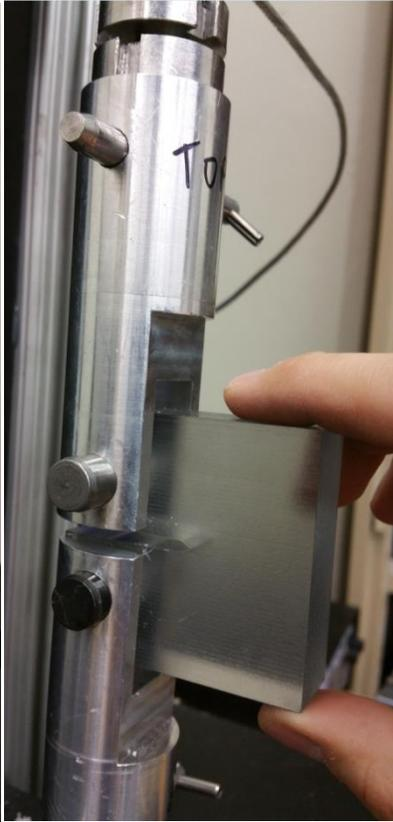
Use your fingers to align the specimen, **make sure you can rotate up and down easily**
