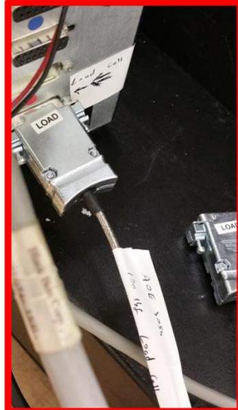
▶ Make sure 100 lbf Force Transducer is connected to MTEST Quattro Unit as shown.
